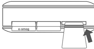
Take the device out of its packaging and place it on a clean and level surface so that it is stable. Unpack the “e-smog” sinus Converter. Insert the sinus Converter straight into the opening on the front of the device and push it in until it stops. Important: The sinus Converter must be plugged into the device with the three golden strips facing upwards. If you have placed the sinus Con-
