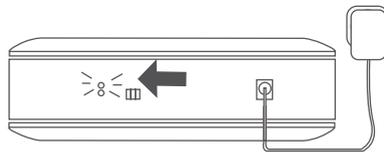
Take the power supply and plug one end into the back of the Room-Converter Plus and the other end into the plug socket. As soon as the Room-Converter Plus is connected to the mains power, it is activated. This is indicated by a green light on the back of the housing. To switch off the Room-Con-
